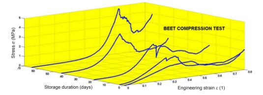
Fig. 3. Stress-strain curves during the storage period.
