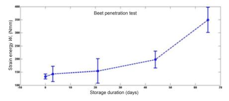
Fig. 8. Effect of the storage duration on the work up to the rupture point.
