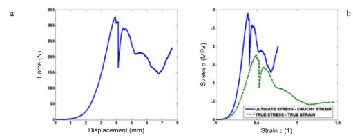
Fig. 2. Example of the experimental record: a – force-displacement and b – stress-strain dependence.
